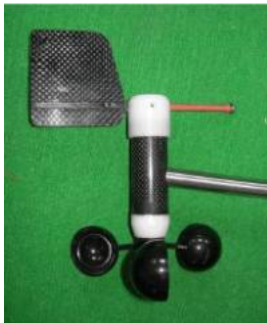
Figure 37: The wind sensor in real [56].
